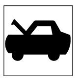
1. Pull the handle with this symbol on it. It is located inside the vehicle on the lower left side of the instrument panel.
